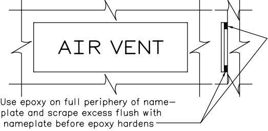
TYPICAL MOUNTING ON CONCRETE WALL
