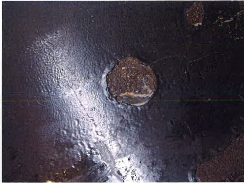
Figure 5. Helium Siphon 40-inch Steel Coal Tar Pipeline Corrosion in 2002
