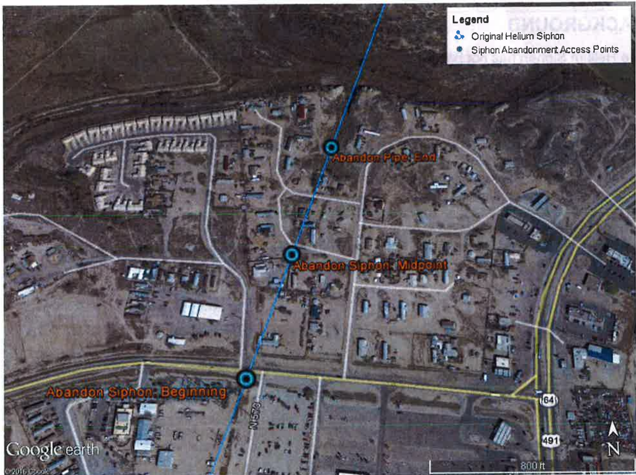
Figure 2. Helium Siphon Section to be Filled with Cellular Concrete
