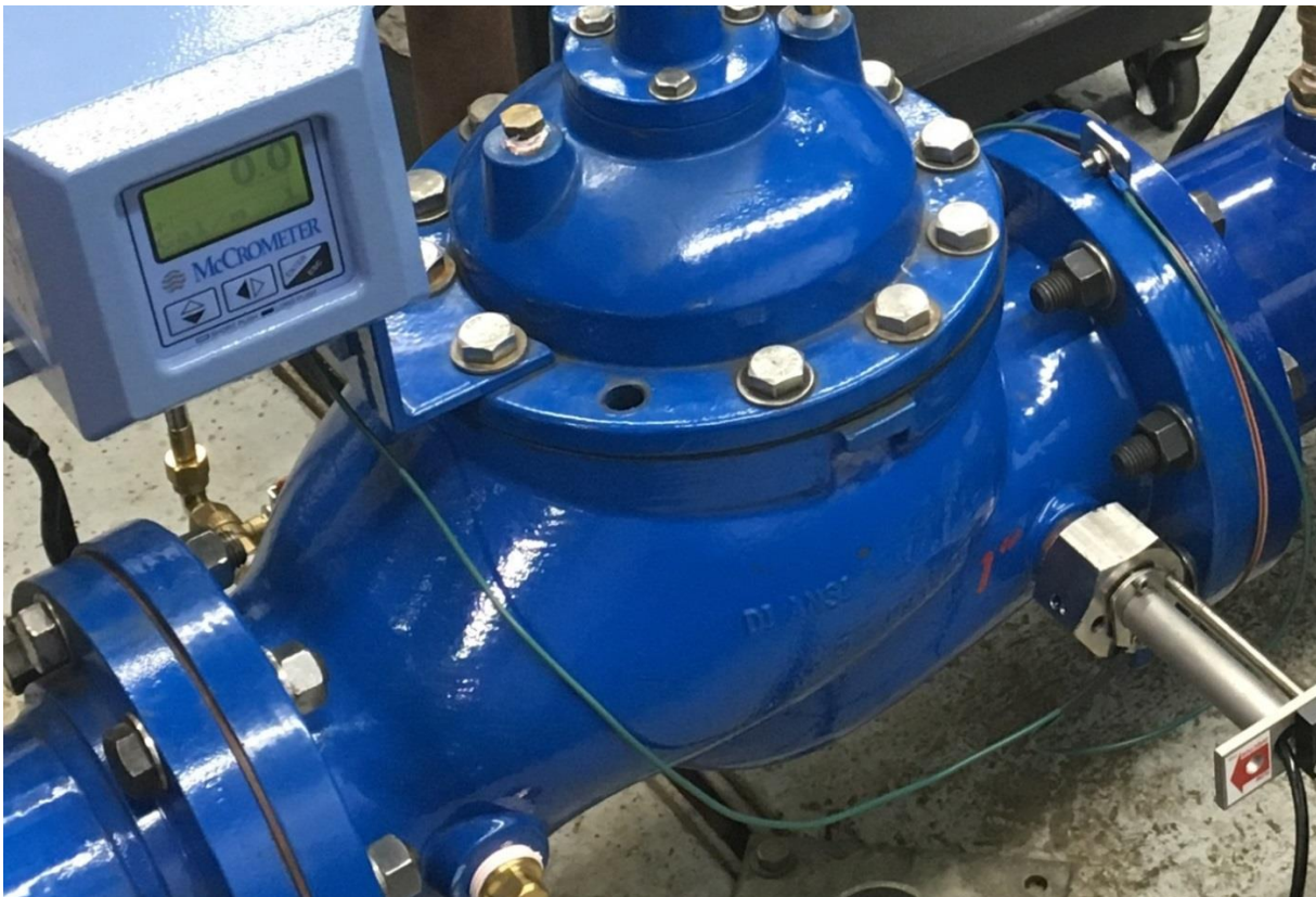
Figure 26: Converter & probe with ground wiring
