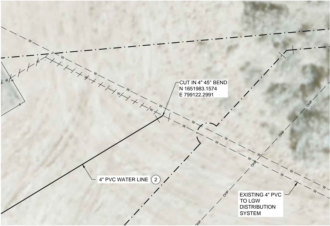
LOWER GREASEWOOD WTP PIPE CONNECTION DETAIL C C-102 SCALE: 1" = 5'
