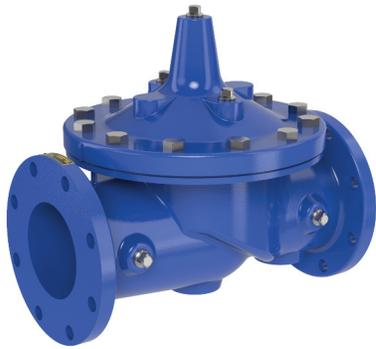
The Cla-Val Model 100-01KO Anti-Cavitation Hytrol Valve is designed for applications where there is a high potential for damage from cavitation. Specify this valve series for a wide variety of control valve applications having pressure differentials up to 300 psid or for relief valves having atmospheric discharge up to 150 psid.
