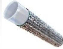
When high temperature performance and excellent chemical compatibility are demanded, Parker 919 PTFE Hose accepts the challenge. This medium pressure hose can withstand temperatures up to 450°F (232°C). A smooth bore natural PTFE core tube and stainless steel braided wire reinforcement tackle corrosive chemicals and abrasive environments.
