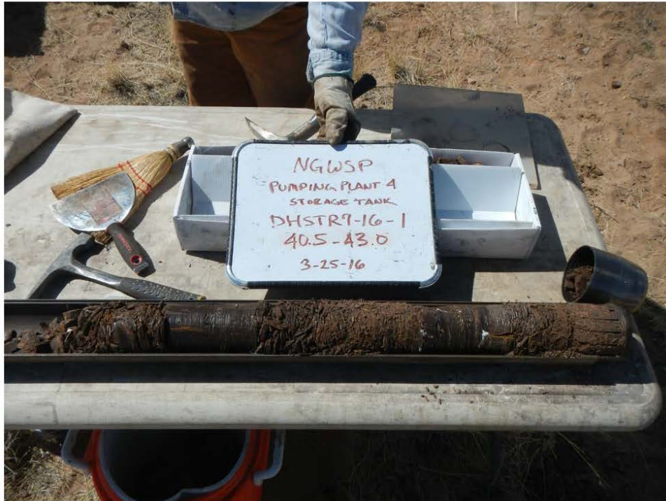
Typical shale and claystone units of the Menefee Formation recovered from drill holes. Image for reference only. Photo taken on 4/14/2016 by C. Beyer.
