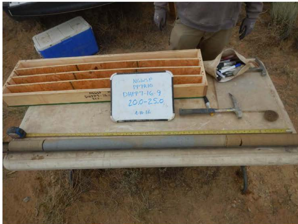
Fine grain sandstone core colored tan, light brown and gray recovered from DHPP7-16-9. Image for reference only.
