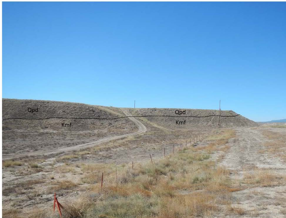
Illustration of the geologic units as they are observed looking south in subsurface investigations. Image for reference only.
