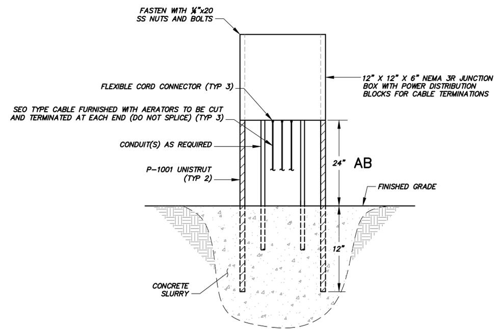
**JB1 TYP** ABOVE GROUND JUNCTION BOX WITH FOUNDATION MOUNTING DETAIL
