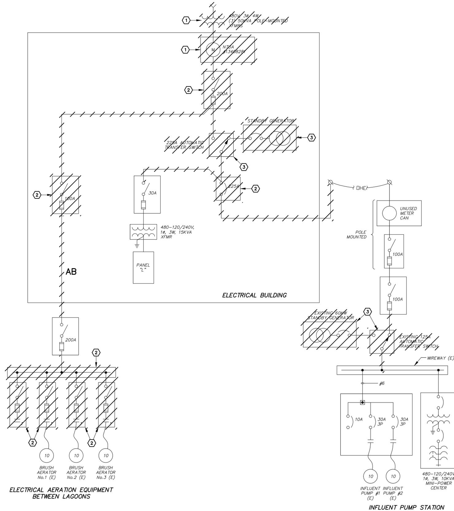
**MAIN PLANT SINGLE LINE DIAGRAM DEMOLITION**
