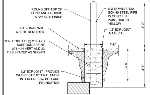
5 TYPICAL STATIONARY BOLLARD DETAIL
