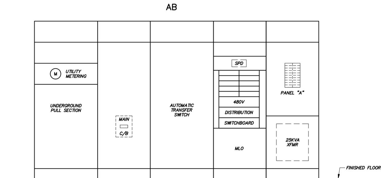
NOTE: FASTEN ELECTRICAL EQUIPMENT TO CONCRETE USING 3/8" GALVANIZED STEEL CONCRETE ANCHORS
