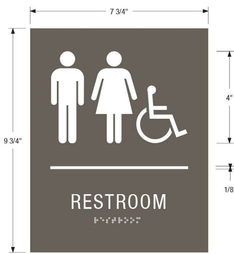
TYPICAL RESTROOM ROOM SIGN SCALE: 1/8" Sign Type: Restroom Room (RR) Basic Sign System Product ID: B10x8 Font: Helvetica Neue Condensed 27 Photogram: 4" Rule: .125" Cap Height: .625" Line Spacing: 150% (.8375") Tactile Lettering: 1/32" Raised, Matte Non Glare Modified Acrylic, White Color Remark (311-201) Sign Face: 1/8" Thick, Matte Non Glare Modified Acrylic, Drift Wood Color Remark (341-595) Mount to Wall: Thick Double Sided Foam Tape & Silicone As Needed
