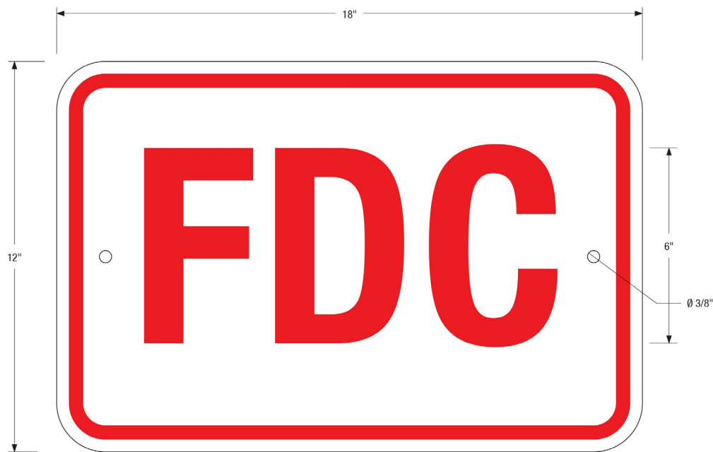
FDC SIGN SCALE: 1/8" Sign Type: FDC Font: Helvetica Neue Condensed 75 Bold Cap Height: 6" Direct To Substrate Digital Printed Graphic: Color Red (CMYK 0 - 100 - 100 - 0) Sign Face: .080" Aluminum, with Reflective Sheeting 3M 4995 White Mount to Wall: Mechanical Fasteners
