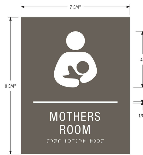
TYPICAL LACTATION ROOM SIGN SCALE: 1/8" Sign Type: Lactation Room (MR) Basic Sign System Product ID: B10x8 Font: Helvetica Neue Condensed 27 Photogram: 4" Rule: .125" Cap Height: .625" Line Spacing: 150% (.8375") Tactile Lettering: 1/32" Raised, Matte Non Glare Modified Acrylic, White Color Remark (311-201) Sign Face: 1/8" Thick, Matte Non Glare Modified Acrylic, Drift Wood Color Remark (341-595) Mount to Wall: Thick Double Sided Foam Tape & Silicone As Needed
