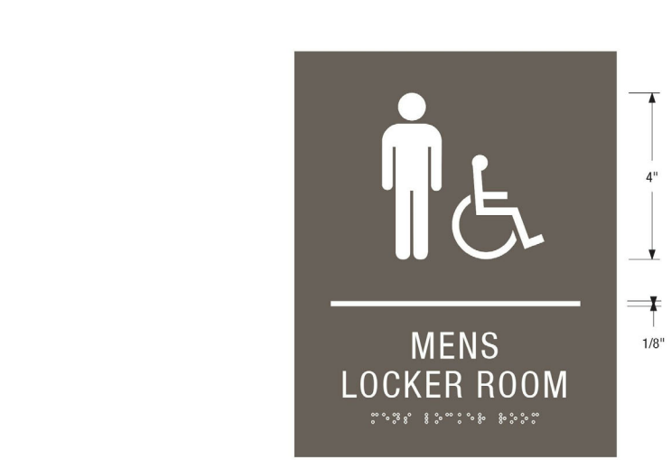
TYPICAL LOCKER ROOM SIGN SCALE: 1/8" Sign Type: Locker Room Sign (LR) Basic Sign System Product ID: B10x8 Font: Helvetica Neue Condensed 27 Photogram: 4" Rule: .125" Cap Height: .625" Line Spacing: 150% (.8375") Tactile Lettering: 1/32" Raised, Matte Non Glare Modified Acrylic, White Color Remark (311-201) Sign Face: 1/8" Thick, Matte Non Glare Modified Acrylic, Drift Wood Color Remark (341-595) Mount to Wall: Thick Double Sided Foam Tape & Silicone As Needed
