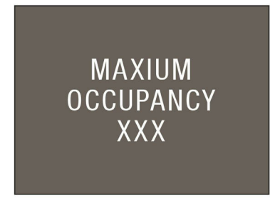
ROOM SIGNS SCALE: 1/8" Sign Type: Room Sign (RS) Basic Sign System Product ID: B6x8 Font: Helvetica Neue Condensed 27 Cap Height: .625" Line Spacing: 150% (.8375") Tactile Lettering: 1/32" Raised, Matte Non Glare Modified Acrylic, White Color Remark (311-201) Sign Face: 1/8" Thick, Matte Non Glare Modified Acrylic, Drift Wood Color Remark (341-595) Braille: NA
