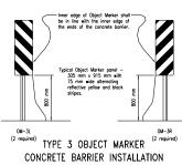
NOTE: If placement between concrete barrier and first timber post is not possible, place between first and second timber post.
