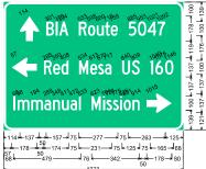
"BIA Route 5047", C 2K 75% spacing; Arrow Custom - 178mm 180", "Red Mesa US 180", C 2K 75% spacing; "Immanual Mission", C 2K 76% spacing; Arrow Custom - 178mm 0",
