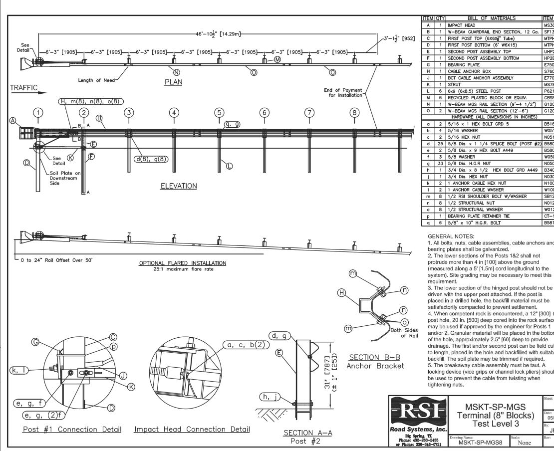
B58 W05 N05 1 3/4 Dia. x 8 1/2 HEX BOLT GRD A449 B340 N03 N10 W10 m 8 1/2 RSI SHOULDER BOLT W/WASHER SB1 N01 W01 CT-1 B58 1. All bolts, nuts, cable assemblies, cable anchors and 2. The lower sections of the Posts 1&2 shall not protrude more than 4 in [100] above the ground
