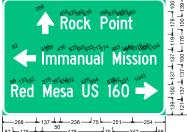
55mm Radlus, 14mm Border, White on, Green, Arrow Custom - 178mm 90; "Rock Point", C 2K 75% spacing; Arrow Custom - 178mm 180; "Immanual Mission", C 2K 75% spacing; "Red Mesa US 160", C 2K 75% spacing; Arrow Custom - 178mm 0;
